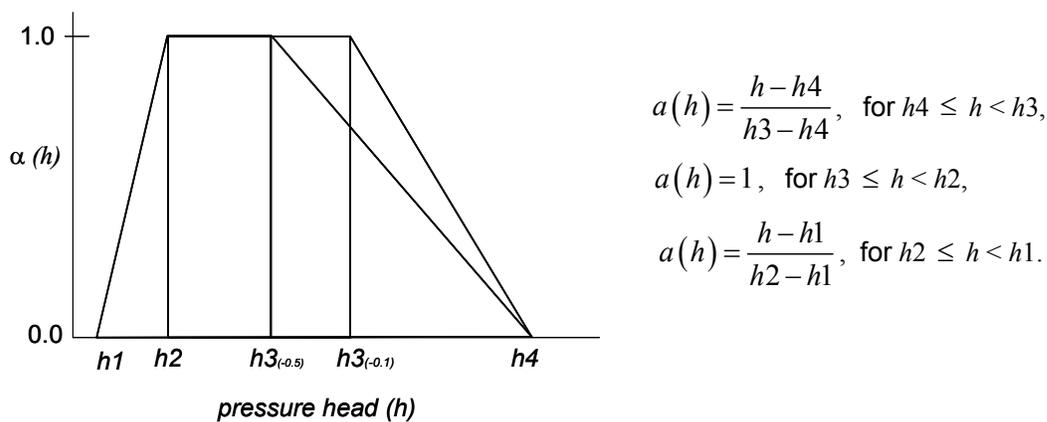
Figure 3: Reduction function  $\alpha(h)$  versus pressure head ( $h$ ).
